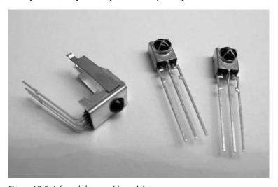
Figure 12-5: Infrared detector/demodulators
