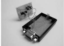
Figure 12-11: Two prototypes for an infrared remote receiver
