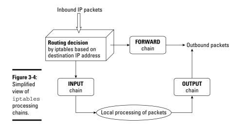
If the kernel has IP forwarding enabled and the packet has a destination IP address of a different network, the kernel passes the packet to the FORWARD chain. If the packet satisfies the rules in the FORWARD chain, it's sent out to the other network. If the kernel does not have IP forwarding enabled and the packet's destination address is not for this server, the packet is dropped.
