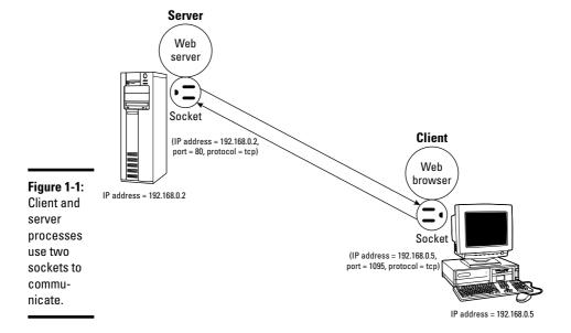
The sequence of events in socket-based data exchanges depends on whether the transfer is connection-oriented (TCP) or connectionless (UDP).
