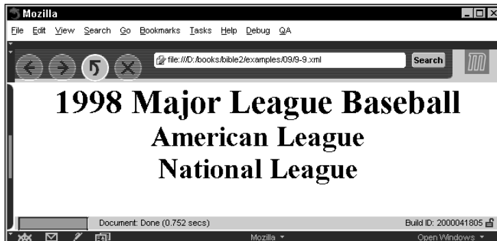
Figure 9-2: A valid document that contains a style sheet, a YEAR element, and two LEAGUE children.
