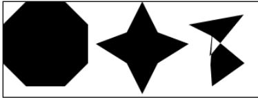
Figure 25-11: A concave polygon, a convex polygon, and a complex polygon, each formed from eight points
