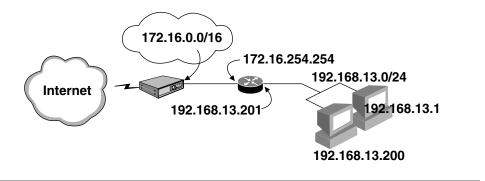
Exhibit 7-12. Isolated internal network supported by a router.
