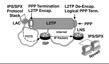
Exhibit 2-17 L2TP connection where the LAC is provided by client software loaded on the laptop.
