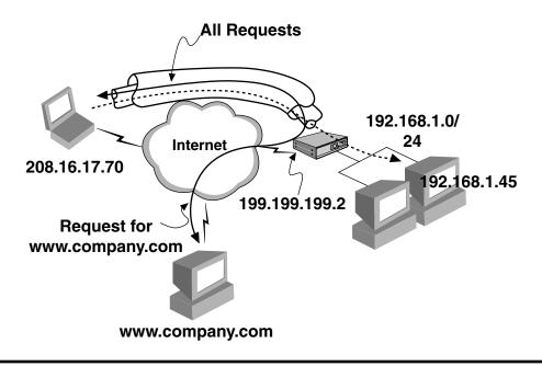
Exhibit 7-19. VPN providing access to the internal network and the Internet through only the VPN.
