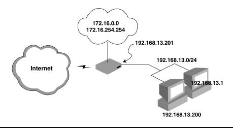
Exhibit 7-13. Security gateway acting as a router for a virtual network.
