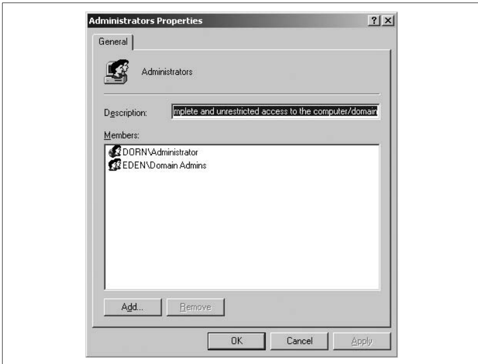
Figure 10-4. Local Administrators group on a Windows XP client containing Domain Admins group
