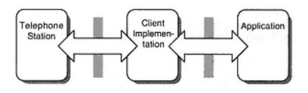
Figure 6-16 Direct-connect example CTI components
