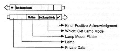
Figure 6-29 Positive acknowledgment sequence example
