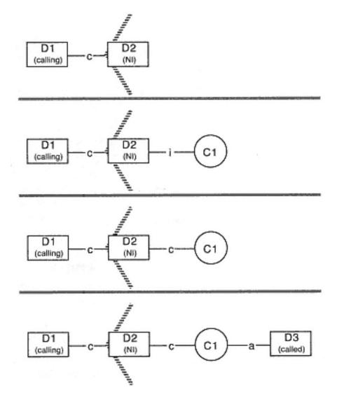
Figure 5-15 Direct inward system access (DISA)
