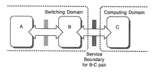
Figure 6-13 Service boundary defines switching domain and computing domain
