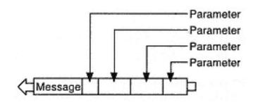
Figure 6-4 Parameters in a CTI message
