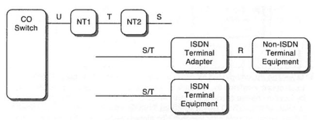
Figure 8-24 ISDN BRI interface points and equipment
