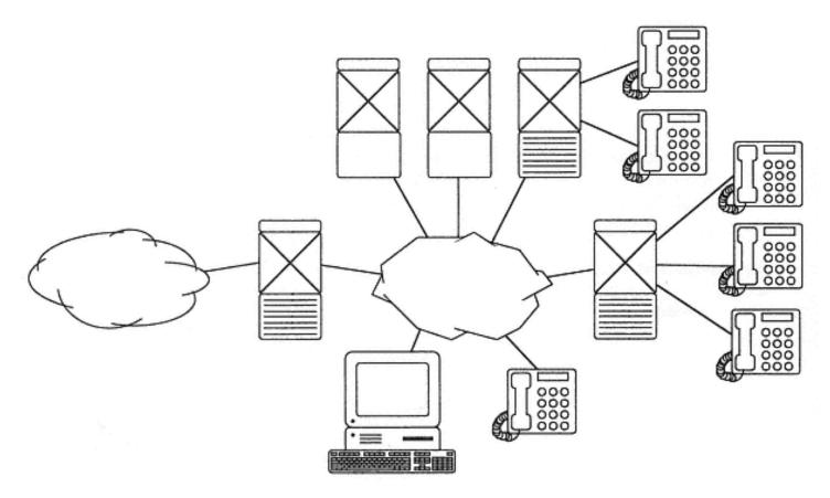
Figure 8-14 Converged backbone network
