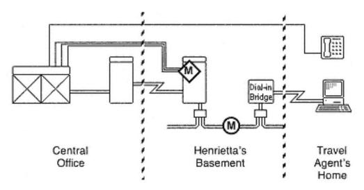
Figure 13-16 Call center solution scenario configuration
