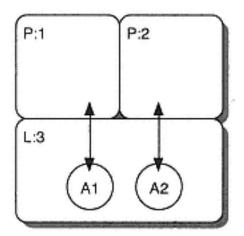
Figure 4-29 Bridged device configuration for a logic device element
