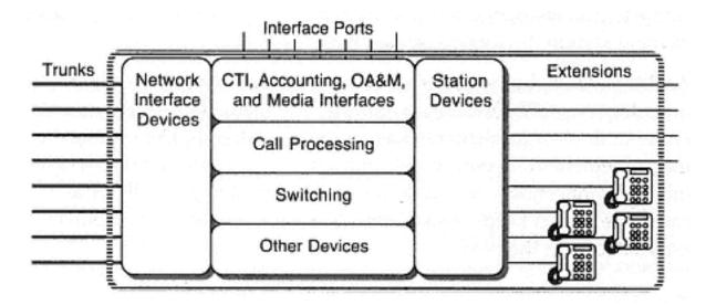
Figure 3-34 Generic telephone switch
