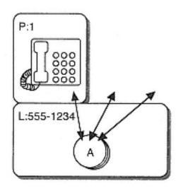
Figure 10-8 Bridged POTS line station example
