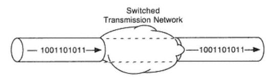
Figure 8-31 Circuit switched network
