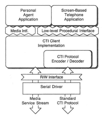
Figure 13-10 Personal telephone agent solution scenario software
