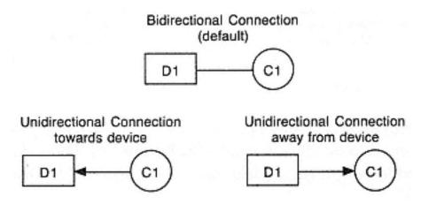
Figure 3-23 Directional connections
