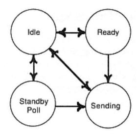
Figure 7-20 Fax sender resource state model
