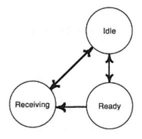
Figure 7-21 Fax receiver resource state model
