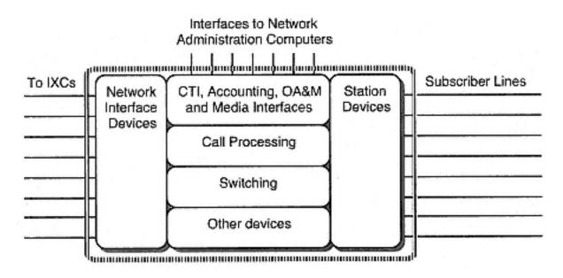
Figure 3-37 A LEC's telephone network
