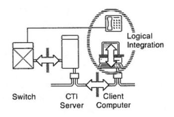
Figure 6-17 Service boundaries in a client-server configuration
