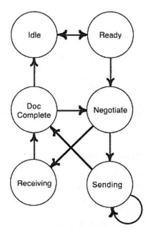
Figure 7-19 Fax low level resource state model
