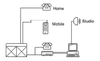
Figure 13-9 Personal telephone agent solution scenario configuration
