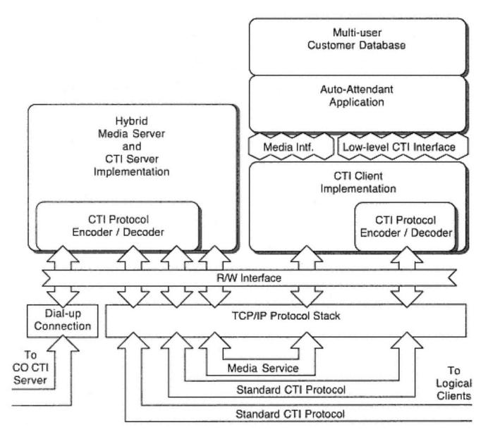
Figure 13-17 Call center solution scenario server software
