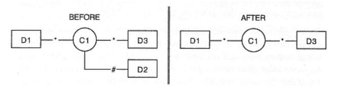
Figure 3-30 Representation of the Clear Connection<sup>3-15</sup> call control service (applied to D2C1)
