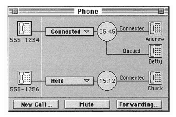
Figure 12-22 Direct manipulation/visualization design approach
