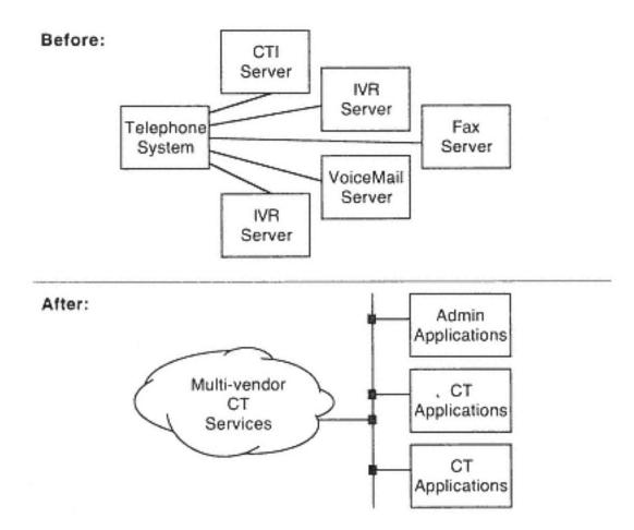
Figure 2-4 Before and After: Scalability of modular telephone systems
