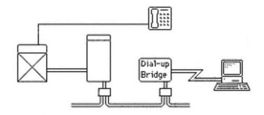
Figure 11-47 LAN remote access configuration
