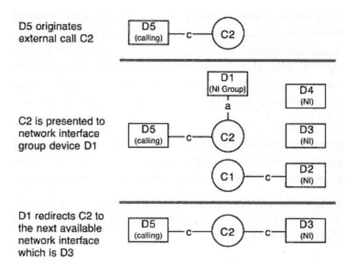
Figure 5-9 Network interface device group behavior
