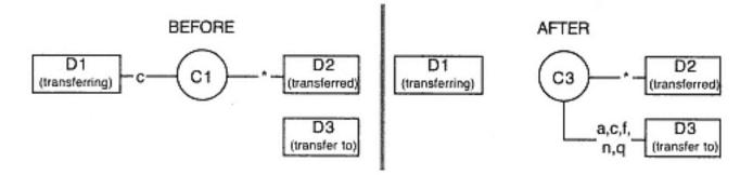
Figure 5-41 Single Step Transfer Call service
