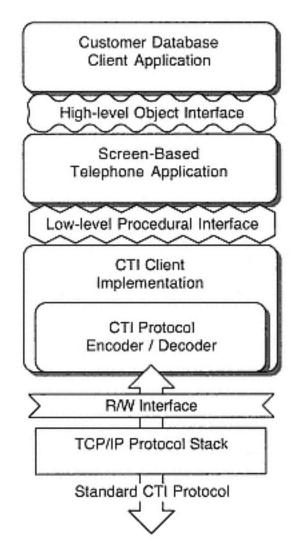
Figure 13-18 Call center solution scenario client software
