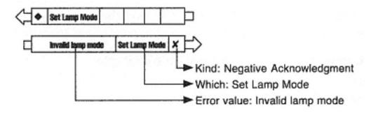
Figure 6-28 Negative acknowledgment sequence example
