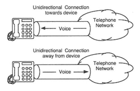
Figure 3-11 Directional connections
