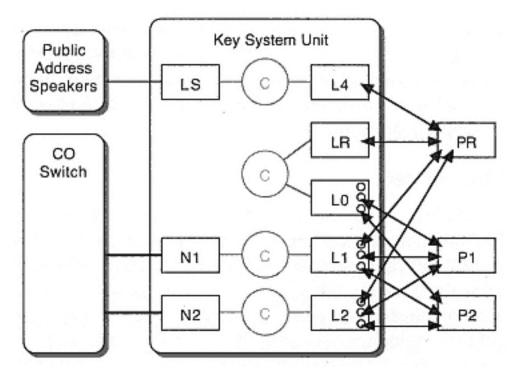
Figure 10-4 Example key system with attendant button and PA system access
