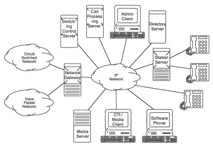
Figure 10-27 Fully modularized iPBX
