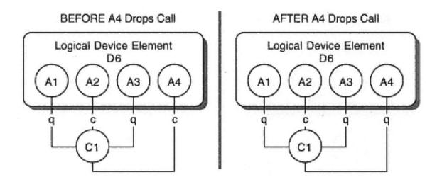
Figure 4-20 Shared–bridged behavior: dropping an appearance
