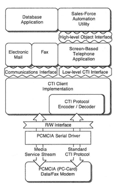
Figure 13-4 Mobile CTI solution scenario software
