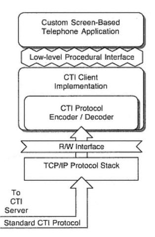
Figure 13-6 Predictive dialing solution scenario software
