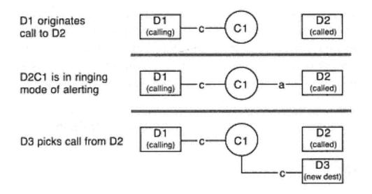
Figure 5-31 Directed Pickup Call for an alerting device
