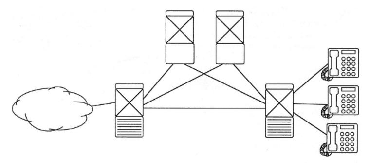
Figure 8-13 Distributed switching function
