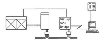
Figure 11-52 CO-server remote access configuration using SVD dial-up bridge
