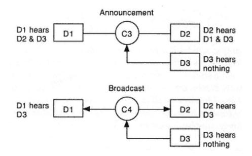
Figure 3-27 Multi-point with unidirectional stream away from device
