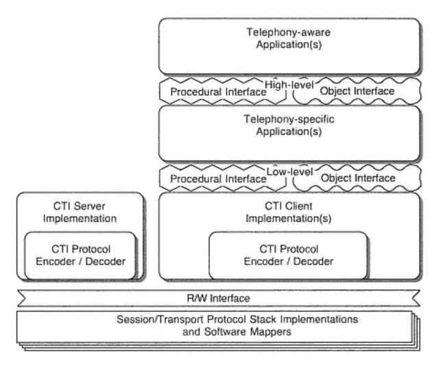
Figure 12-2 CTI software component framework
