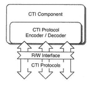
Figure 11-11 CTI component using CTI protocols
