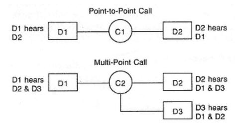
Figure 3-25 Point-to-point and multi-point calls
