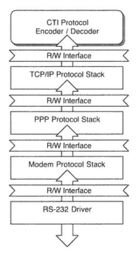
Figure 12-8 Example of layering with R/W interfaces
