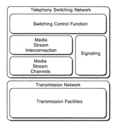
Figure 3-7 Telephony switching fabric
