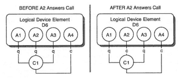
Figure 4-19 Shared–bridged behavior: adding a second appearance
