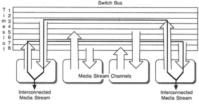
Figure 8-8 Switch bus architecture
