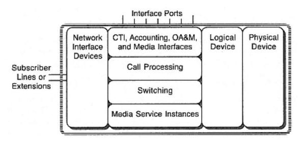
Figure 3-36 Generic telephone station modeled from station's perspective
