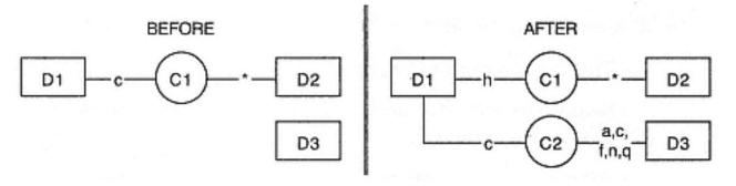
Figure 3-29 Switching service representation in terms of "before" and "after"
