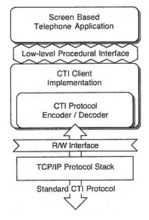
Figure 13-21 IP telephone system solution scenario client software
