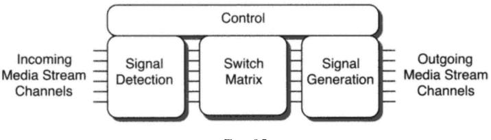
Figure 8-7 Switch matrix implementation
