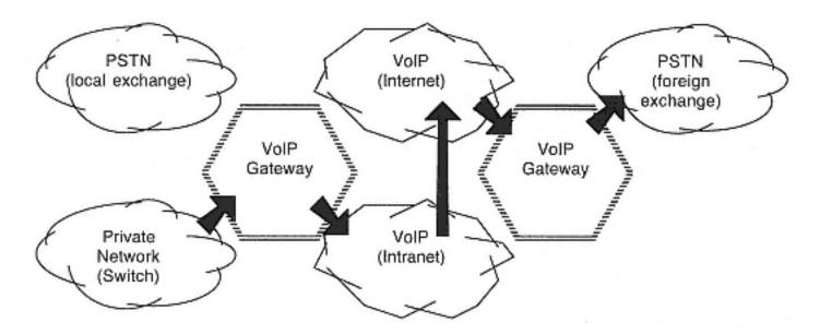
Figure 10-25 Using Internet telephony for FX lines
