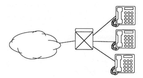
Figure 8-12 Traditional telephone switch
