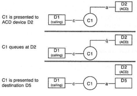
Figure 5-19 Non-visible ACD model
