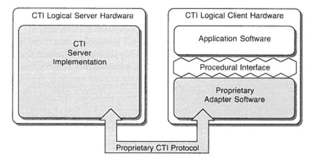
Figure 11-9 Proprietary CT protocol with adapter software
