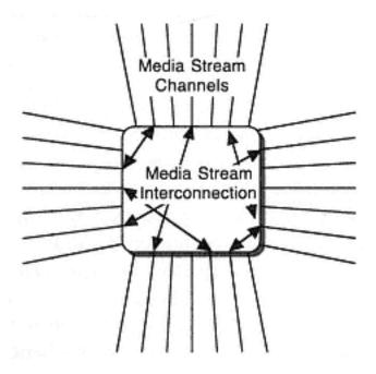
Figure 8-2 Media stream interconnection is a logical hub
