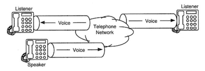
Figure 3-15 Three-point call with broadcaster and listeners
