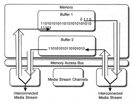
Figure 8-9 Memory-based switching
