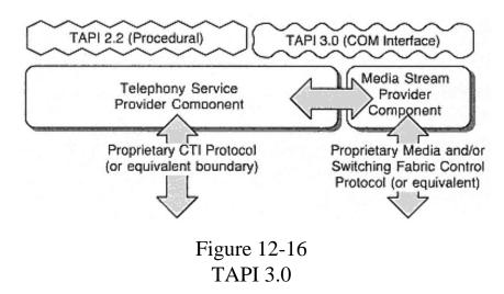
The most significant improvement in TAPI 3.0 is that it provides access to an object that corresponds to a call. Microsoft refers to this object as a *call hub*. The call hub object allows an application to enumerate the other connections associated with the call and examine their states independently. Though the labels are different, the TAPI 3.0 object model, illustrated in Figure 12-17, reflects the standard CTI object model.
