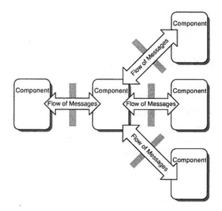
Figure 6-8 Fan-out component
