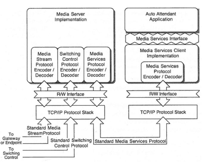
Figure 13-22 IP telephone system solution scenario media services software
