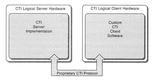
Figure 11-8 Custom CT solution using proprietary CT protocol
