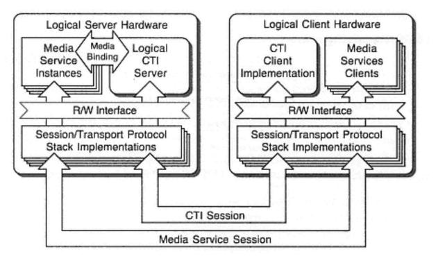
Figure 6-34 Media stream binding model
