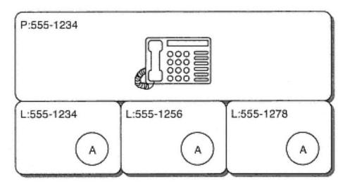
Figure 10-11 Multiple line station example
