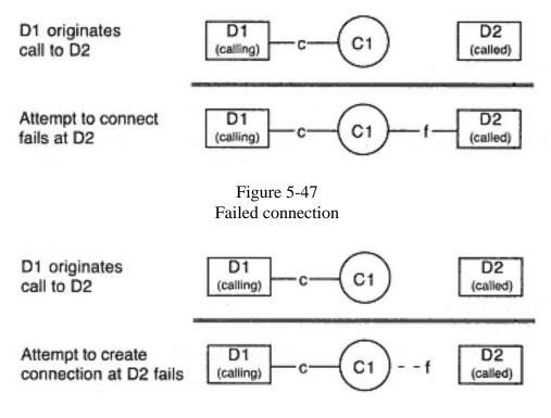
Figure 5-48 Failed connection attempt (failed call)
