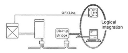
Figure 11-48 LAN remote access configuration with OPX
