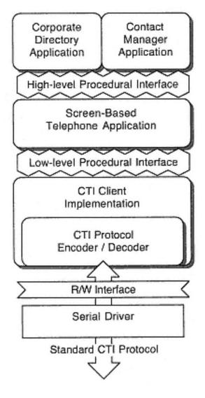
Figure 13-2 Screen-based telephony solution scenario software
