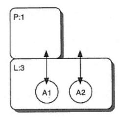
Figure 4-30 Bridged device configuration: for a physical device element
