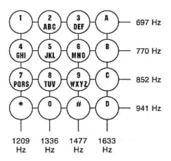
The first three columns represent the twelve DTMF tones in widespread use. The last column represents four additional DTMF tones labeled "A" through "D" which are generally referred to as military or autovon tones. These additional tones should not be confused with the alphabetic labeling found on most telephone dial pads.
