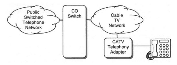
Figure 8-29 Cable TV network providing subscriber loop
