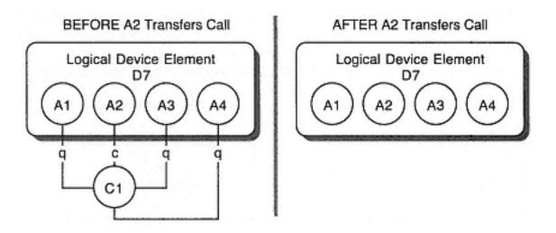
Figure 4-22 Independent–shared–bridged behavior: only A2 is active
