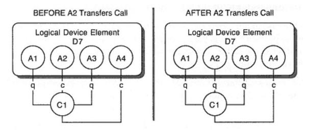
Figure 4-21 Independent–shared–bridged behavior: A2 and A4 active
