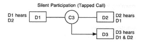
Figure 3-26 Multi-point with unidirectional stream towards device
