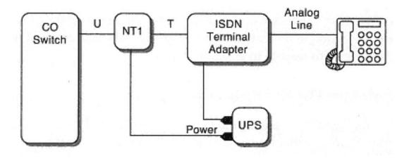
Figure 8-26 Analog stations on an ISDN line
