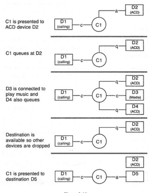
Figure 5-18 Visible ACD-related devices model
