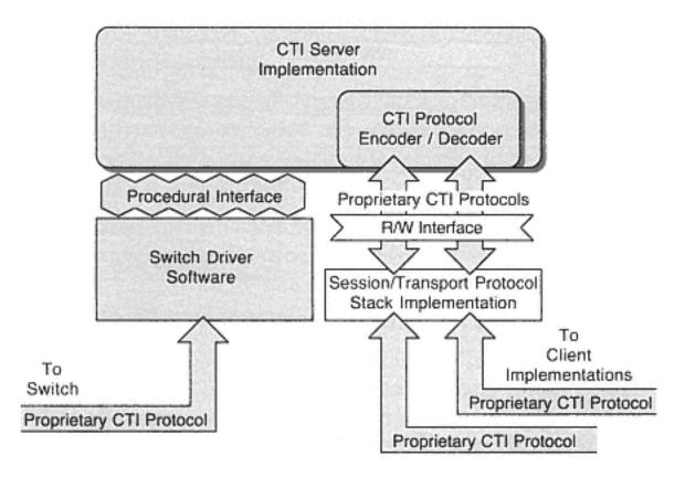
Figure 12-5 CTI server implementation with proprietary interfaces
