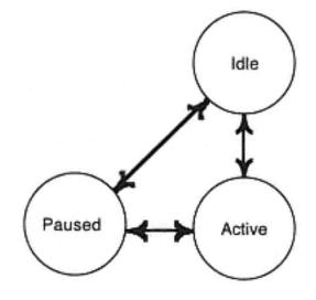
Figure 7-17 Recorder resource state model
