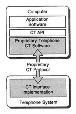
Figure 1-10 The second phase: API layering
