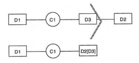
Figure 4-9 Network interface device representation
