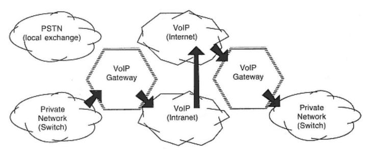
Figure 10-24 Using Internet telephony for tie lines
