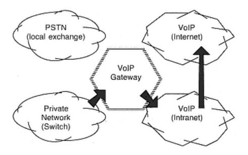
Figure 10-26 Using Internet telephony for OPX lines
