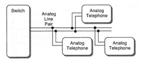
Figure 8-17 Analog local loop with bridged telephone stations
