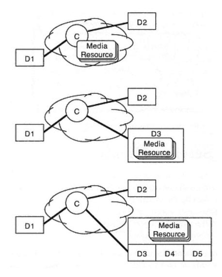
Figure 7-3 Media access devices and media binding
