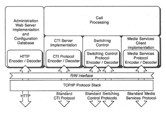
Figure 13-20 IP telephone system solution iPBX software components
