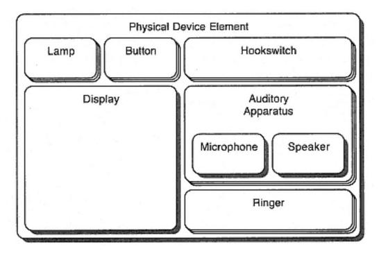
Figure 4-2 Physical device element components
