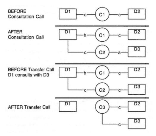
Figure 5-40 Two-step transfer call sequence
