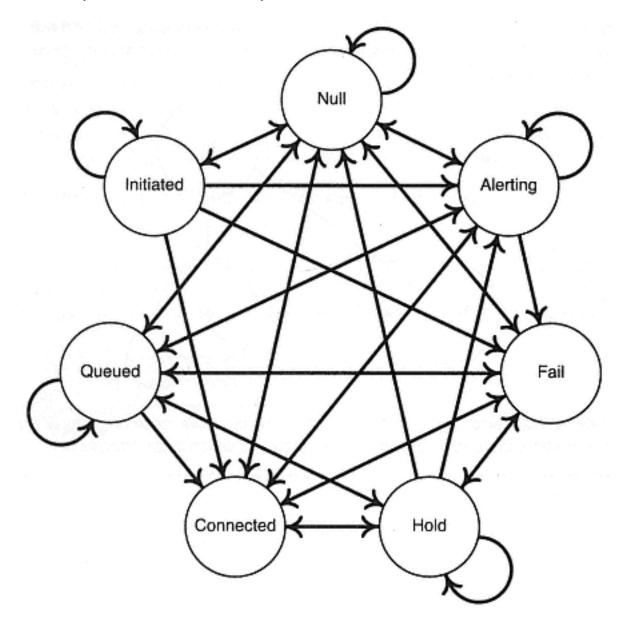
Figure 3-16 Connection state diagram
