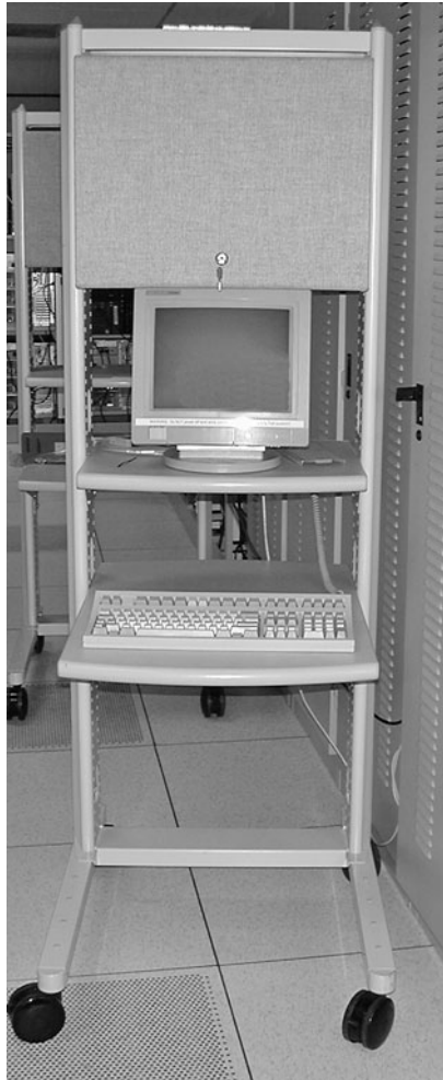
Figure 6.15 Synopsys has several serial console carts that can be wheeled up to a machine if the main console server fails or if the one machine with a head in the machine room is in use.
