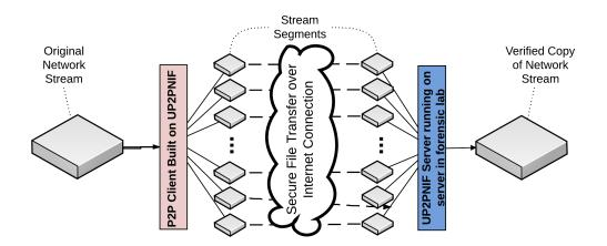
Figure 5.4: Overview of UP2PNIF evidence transmission architecture. This diagram shows the remote transmission from the UP2PNIF framework X = number of segments to transfer entire network stream.
