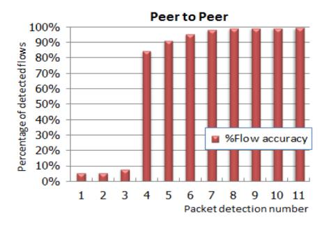
Figure 3.9: Flow accuracy results for P2P traffic as a function of the packet detection number
