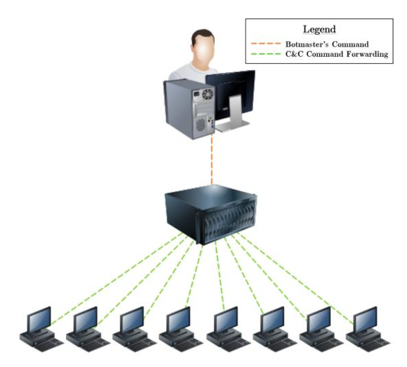
Figure 4.4: Command and Control Server Botnet Network Architecture
