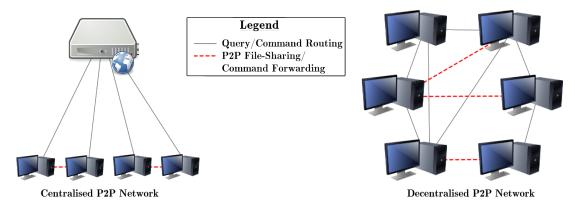
Figure 5.1: A Comparison of Centralised (left) and Decentralised (right) P2P Network Architectures.
