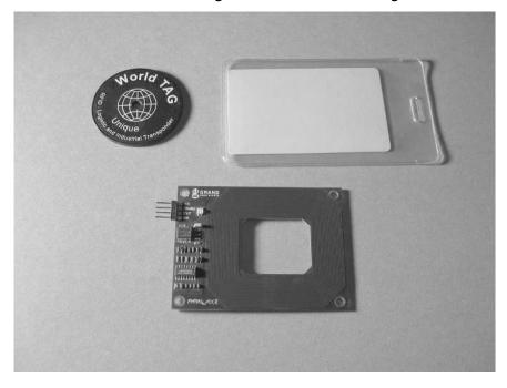
Figure 1.3 Two Different RFID Tags and Reader with Integral Antenna
