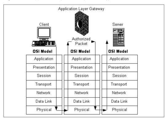
Figure 6.12 Application Layer Gateway Technology
