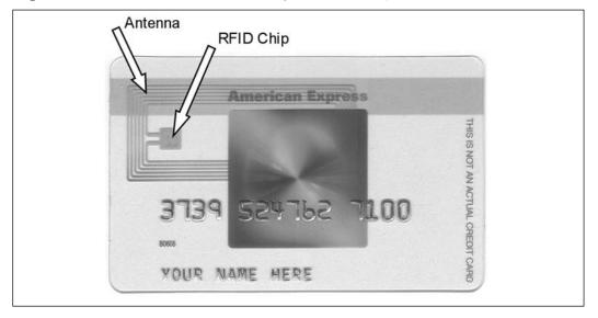
Figure 1.7 Fake Credit Card Showing the RFID Chip and Antenna
