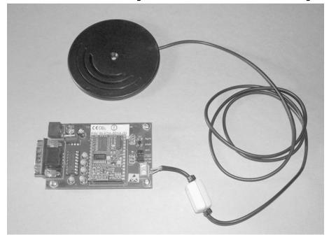
Figure 1.2 RFID Reader Including the Antenna and Electronics Package
