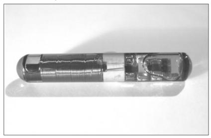
Figure 1.8 A Passive Tag's Internal Components
