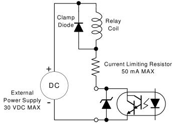
In this example, a relay coil is being driven. The current through the coil needs to be limited to 50 mA or less, which is accomplished by selecting an appropriate value of current limiting resistor.
