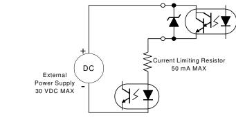
An opto isolator is being driven in this example. The current through the output needs to be limited to 50 mA or less, which is accomplished by selecting an appropriate current limiting resistor. The voltage of the external power source needs to be 30 VDC or less and can be the same source used to provide power to the inputs.
