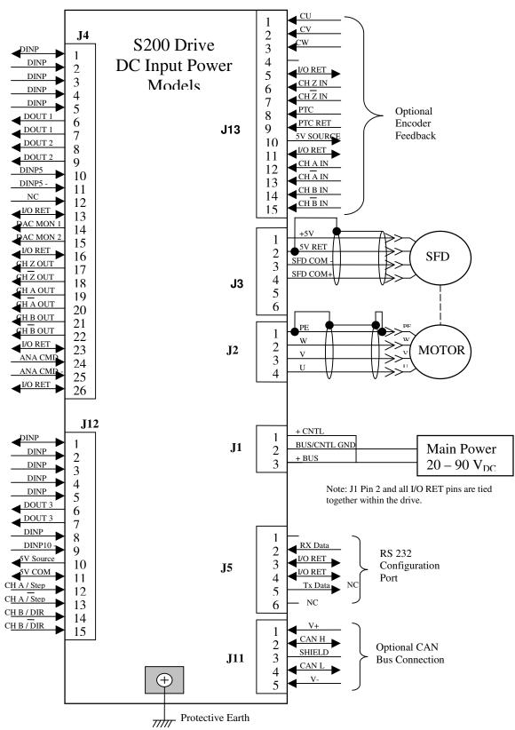
2.4 S200 Position Node DC Drive Wiring Diagram
