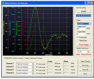
Up to 4 channels of data can be recorded simultaneously. Set the channels for the desired data, the sample rate for an appropriate buffer size, and a trigger level suitable for the capture. Press Start. The scope data plots will be presented after the trigger occurs. It is important to note that each plot has an independent vertical axis scalar.
