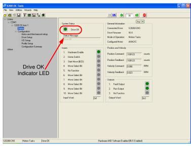
The Status screen can be helpful to understand system operation. Drive Status should read 'OK'. If not then a meaningful fault code will be shown. General information about drive size and firmware version is shown. Energizing a
