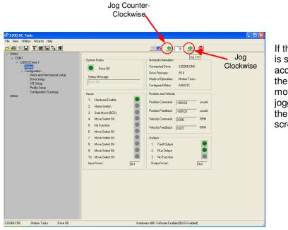
If the system is safe to accept motion then the motor can be jogged from the status screen.
