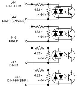
Input current is a function of the input voltage and listed in the following table.
