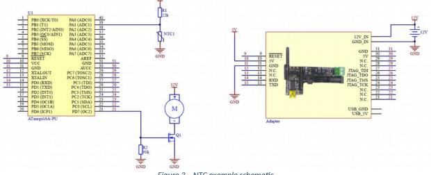
Figure 3 – NTC example schematic
