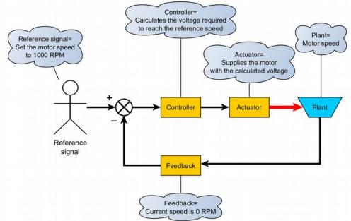
Figure 2 – An example closed-loop block diagram
