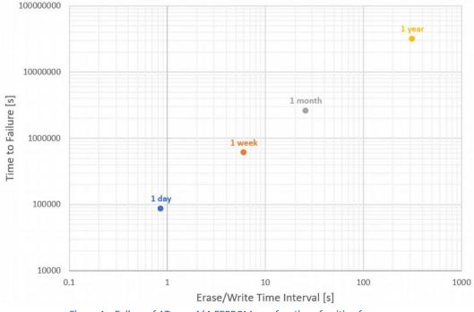
Figure 1 - Failure of ATmega16A EEPROM as a function of writing frequency
