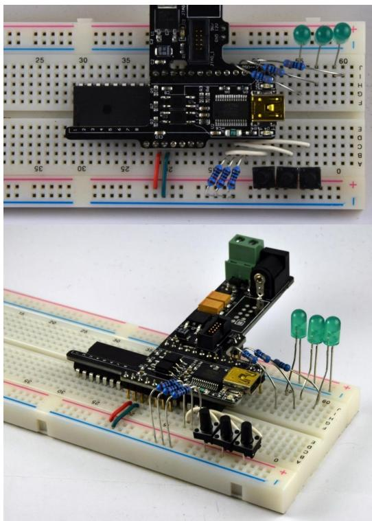
Figure 3 – Assembled example circuit for the EEPROM project
