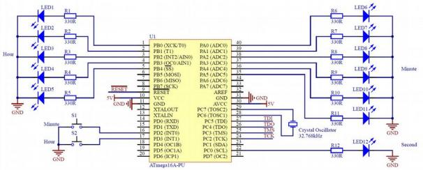
Figure 6 – Schematic of the clock using an external crystal
