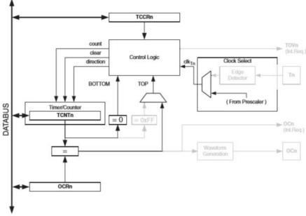
Figure 3 - The internal structure of Timer/Counter0
