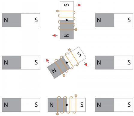
Figure 5 – Force on a magnet/coil
