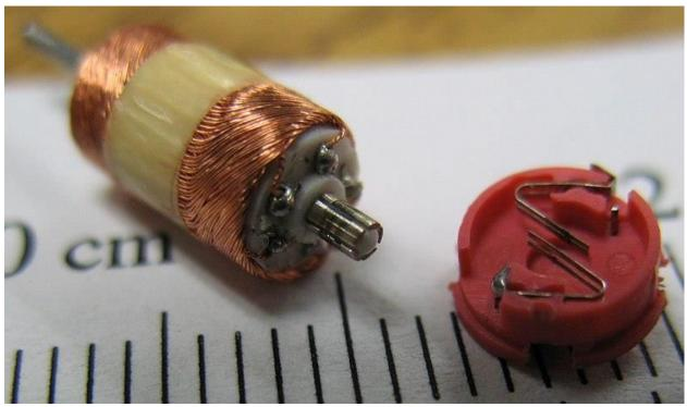
Figure 8 - Commutator Author: Dale Mahaiko [CC BY-SA 3.0 (https://creativecommons.org/licenses/by-sa/3.0)] https://en.wikipedia.org/wiki/File:Tiny\_motor\_windings\_-\_commutator\_-\_brushes\_in\_Zip\_Zaps\_toy\_R-C\_car.jpg
