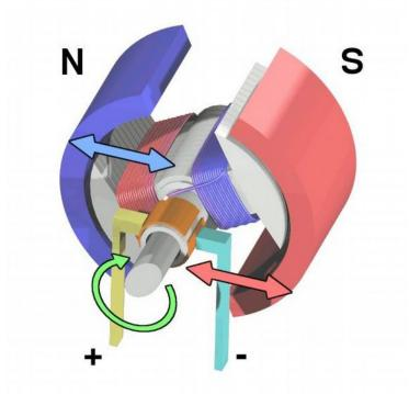
Figure 6 - with the commutator and voltage source. The figure is only for demonstration purposes, in case of this layout, the commutator would short circuit the source by turning Author: Wapcaplet [CC BY-SA 3.0 (<u>https://creativecommons.org/licenses/by-sa/3.0</u>)] <u>http://en.wikipedia.org/wiki/Image:Electric\_motor\_cycle\_3.png</u>
