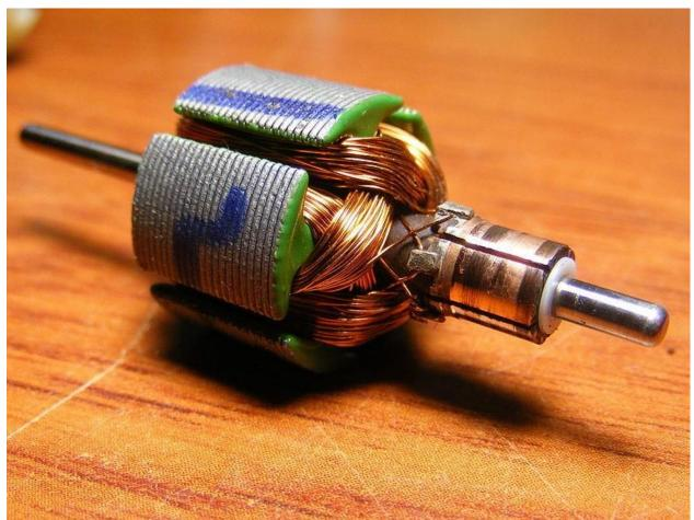
Figure 9 - Commutator Author: Jjmontero9 [CC BY-SA 3.0 (https://creativecommons.org/licenses/by-sa/3.0)] https://commons.wikimedia.org/wiki/File:Small\_DC\_Motor\_Rotor.JPG
