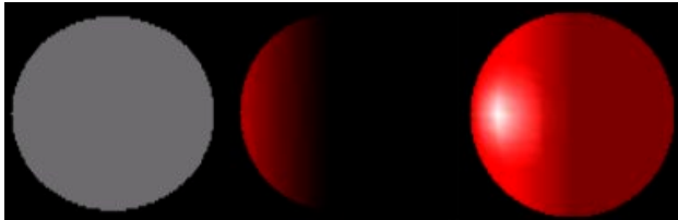
Figure 11–3. Different material/light types. Left: ambient only. Middle: diffuse only. Right: ambient and diffuse with specular highlight.
