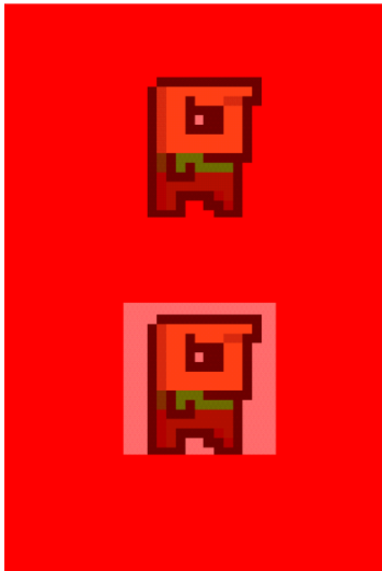
Figure 7-17. An alternative version of RGBA8888 Bob using per-vertex alpha of 0.5f (top of the screen)
