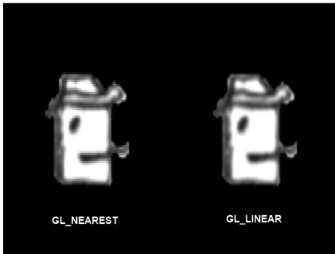
Figure 7-12. GL10.GL_NEAREST vs. GL10.GL_LINEAR. The first filter type makes for a pixelated look; the second one smoothes things out a little.
