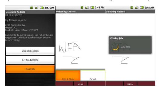
Figure 12.13 The CloseJob Activity capturing a signature and sending data to the server
